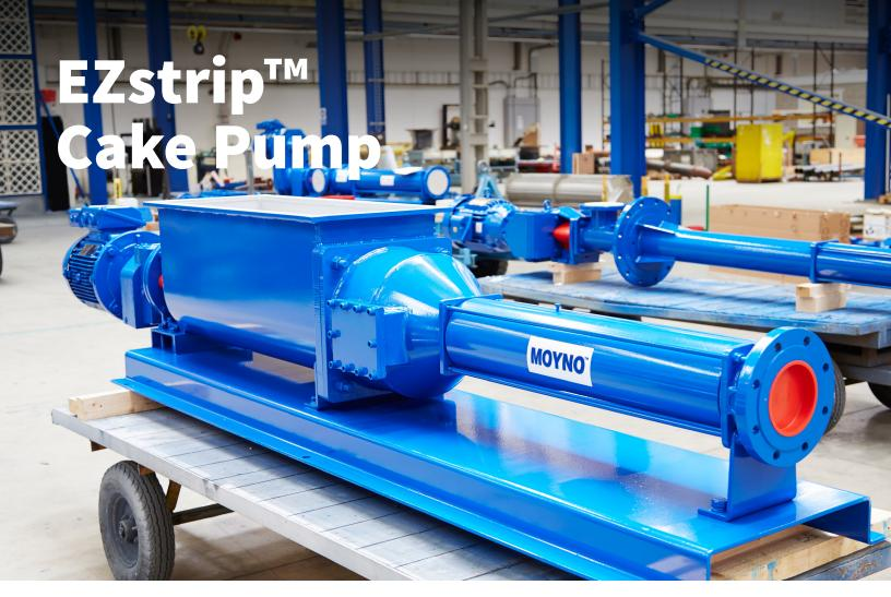
The EZstrip Cake Pump is designed with a large auger inlet and screw conveyor. The screw conveyor extends to the compression area to help push the sludge cake into the cavities of the rotor and stator and provide consistent pumping.
